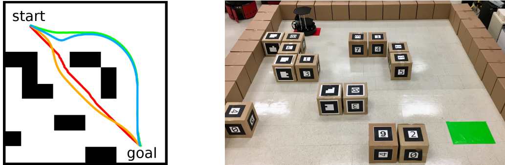
Figure 3.4: The OFFICE map ( left ) with the riskiest path ( red ), a very risky path ( yellow ), a very safe path ( blue ), and the safest path ( green ) in addition to the environment of the mobile robot ( right ).
